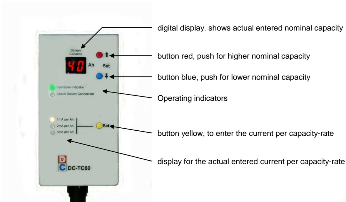
Adjustable for NiCd-batteries up to 60Ah.
